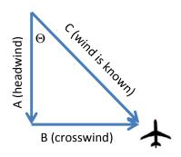
$\Theta$  is known because we know the wind direction. C is known because we know the wind speed. So we use trigonometry to calculate A and B:
