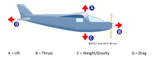
**Lift:** Air flowing over the wings and the angle of the wing relative to the passing air together move the aircraft upward.
