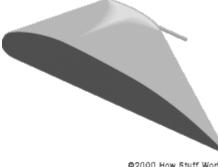
Wings with a steep angle of attack have more drag and more lift. This allows the plane to fly slower.
