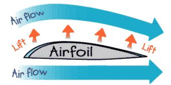
Air moving over the longer distance of the curved upper wing surface must travel faster than the air flowing the shorter distance under the flatter bottom surface of the wing. According to Bernoulli's principle, the difference in the speed of the air, which behaves like a fluid, produces lower pressure above the wing than below it. This pressure difference produces lift.
