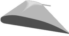
Wings with a shallow angle of attack have less drag but also less lift.
