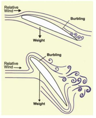
Airflow over a wing in flight, at different angles of attack:
