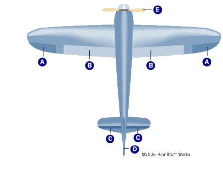
A = Ailerons B = Flaps C = Elevator D = Rudder E = Propeller
